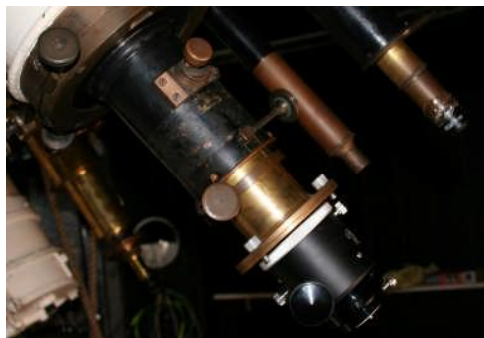
8-inch refractor rotating tail piece showing sliding focus tube and the Crayford 1:10 focuser. Image Tony Cross.
