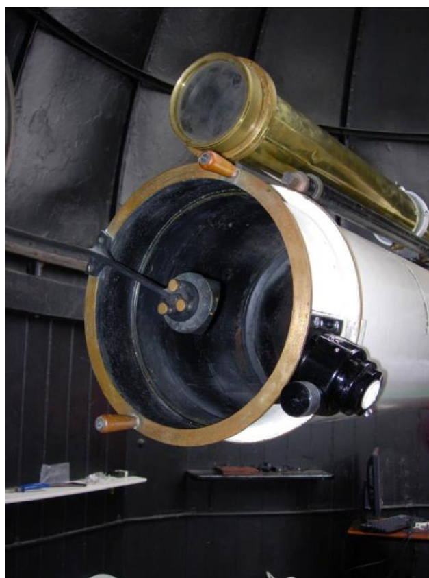
12-inch Newt. showing the Crayford focuser and the 5-inch Wray acquisition scope. Image K J Kilburn
