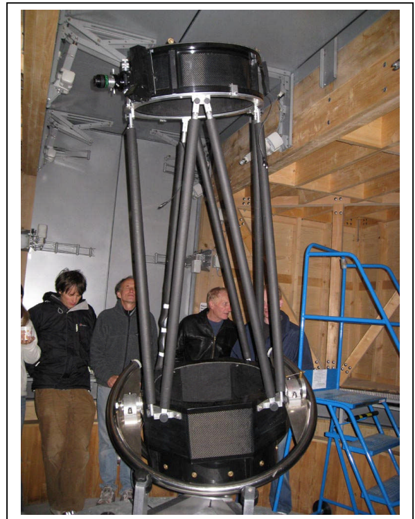
Pulsar optical 20 inch Split-ring Equatorial F4 telescope. Fully manual with potential for camera mount and motor drives for remote operation.
