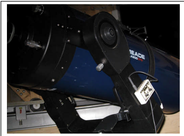
Meade LX200 14 inch Schmidt-Cassegrain with built in GPS and motor drives. Mounted equatorially and wired for computer connection in a warm room
